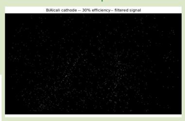
**NB:** framerate is 64 fps. A framerato fo approx 2000 will be used, so the noise will be reduced of at least a factor 100
