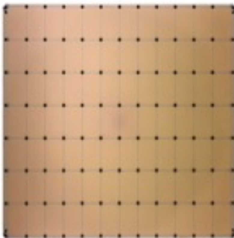
Cerebras WSE-3 4 Trillion Transistors 46,225 mm 2 Silicon
