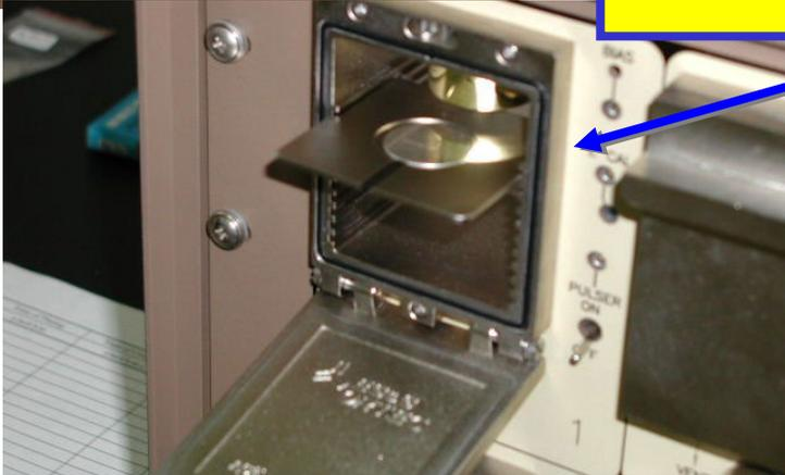
Cyclone® Plus Storage Phosphor System 2D imaging for gamma-beta emitters
