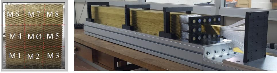
**Figure 1.** View of the prototype and its segmentation in the  $M_0 - M_8$  modules.
