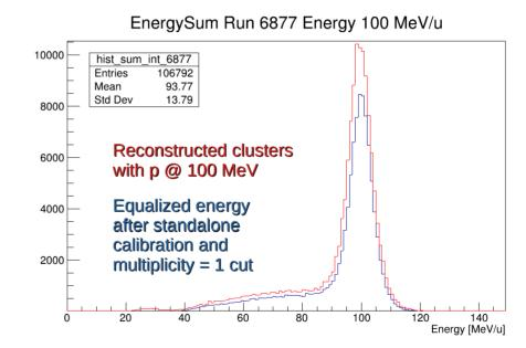
Calibration was tested on CALO clusters reconstructed in shoe, for a calibration run with p @ 100 MeV (6877) >> response and FWHM unmodified with respect to previous, standalone results.
