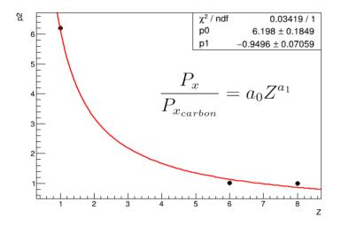
Different crystals  $\rightarrow$  different power-law parameters >> we tried extracting  $a_0$ ,  $a_1$  without He and then reconstructing  $p_0$ ,  $p_1$ ,  $p_2$  for He on **the same crystal**.
