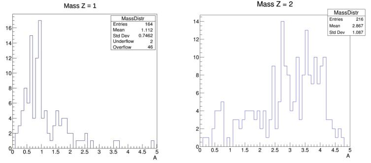
Mass reconstruction for Z = 1 and Z = 2 fragments was attempted by matching CALO clusters with the closest TW hits, by using power-law calibration functions with respect to Z. Note that:
