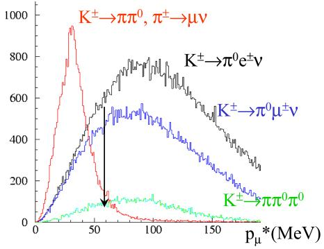
•  $K^{\pm} \rightarrow \pi^{\pm} \pi^{0}$  events are rejected evaluating the missing momentum at the decay vertex, and cutting on momentum of the secondary track in the P<sub>miss</sub> rest frame (p<sub>µ</sub>\*>60 MeV)
