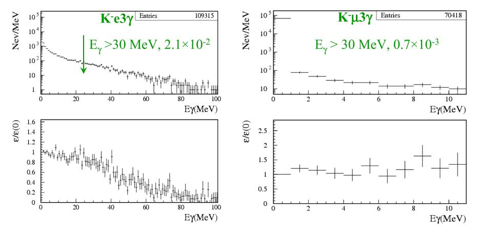
• The acceptance are determined with a generator that uses the soft-photon approximation to sum the amplitudes for real and virtual processes to all orders of  $\alpha$  (C.Gatti, *Eur.Phys. J. C*, 45417, 2006).
