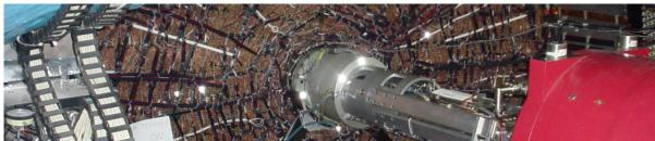
$\begin{array}{l} \mbox{He/IsoC}_4 \mbox{H}_{10} \ 90/10 \ drift \ chamber \\ \mbox{4m-}\ensuremath{\varnothing}, \ 3.75m\mbox{-length}, \ all\mbox{-stereo} \\ \mbox{\sigma}_p/p = 0.4 \ \% \ (tracks \ with \ \theta > 45^\circ) \\ \mbox{\sigma}_x^{\ hit} = 150 \ \mu m \ (xy), \ 2 \ mm \ (z) \\ \mbox{\sigma}_x^{\ vertex} \ \sim 1 \ mm \end{array}$
