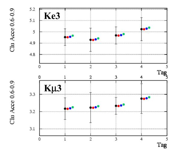
• To check the robustness of the cluster efficiency correction wrt the acceptance cut, vary the opening angle ( $\cos(\theta) > 0.7$ ) and use the CLU correction obtained:  $\cos(\theta) > 0.6$ > 0.8> 0.9
