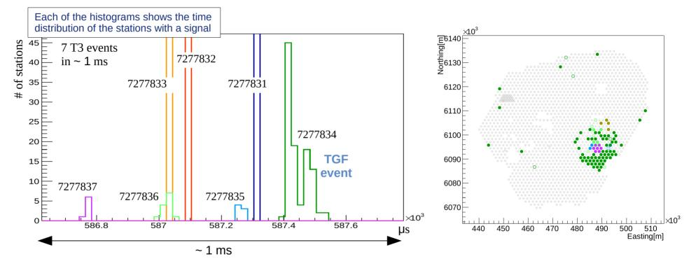
Behaviour similar to the events observed by the Santa Cruz group (J. Ortberg & D. Smith) in Japan and New Mexico: timing consistent with a stepped leader making a connection at that time  $\rightarrow$  the upward return stroke enhances the field in the right direction for the avalanche to be aimed toward the ground with a strong horizontal component (-CG – negative cloud-to-ground).
