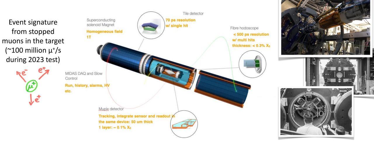
Previous limit (SINDRUM@PSI)  $\mathcal{B}(\mu \rightarrow eee) < 1 \times 10^{-12}$ (90%CL) Mu3e phase I, starting 2026  $\mathcal{B}(\mu \rightarrow eee) \sim 1 \times 10^{-15}$ expected sensitivity (~2030) Mu3e phase II at HiMB,  $10^9 \mu/s$   $\mathcal{B}(\mu \rightarrow eee) \sim 1 \times 10^{-16}$ expected sensitivity(~2035)
