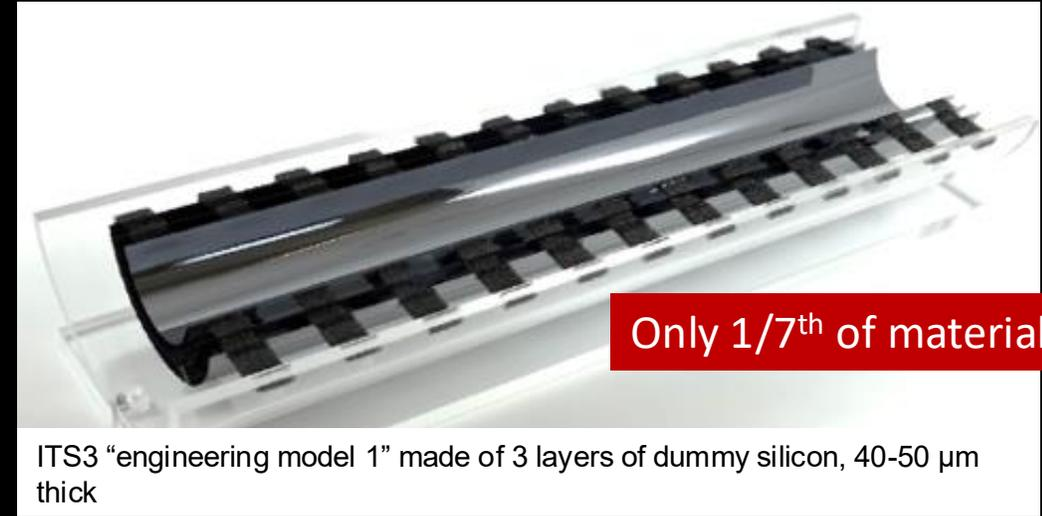
ITS3 "engineering model 1" made of 3 layers of dummy silicon, 40-50  $\mu\text{m}$  thick
