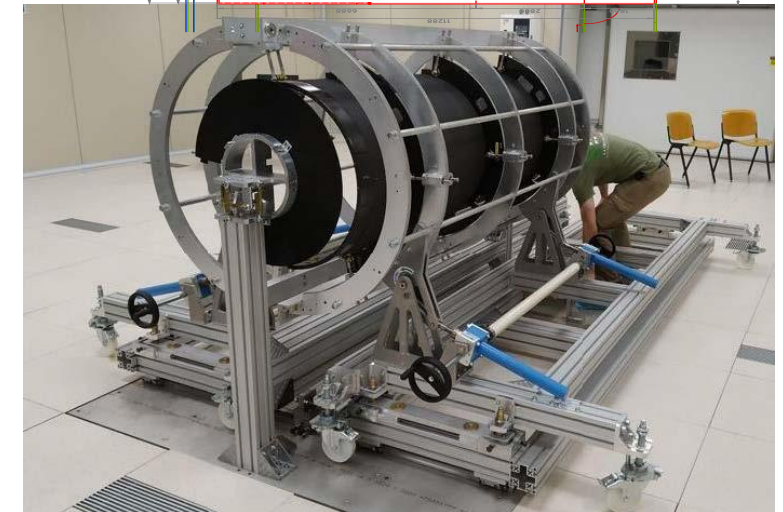
ATLAS ITK Mechanical Support for the integration of the Endcap @LNF
