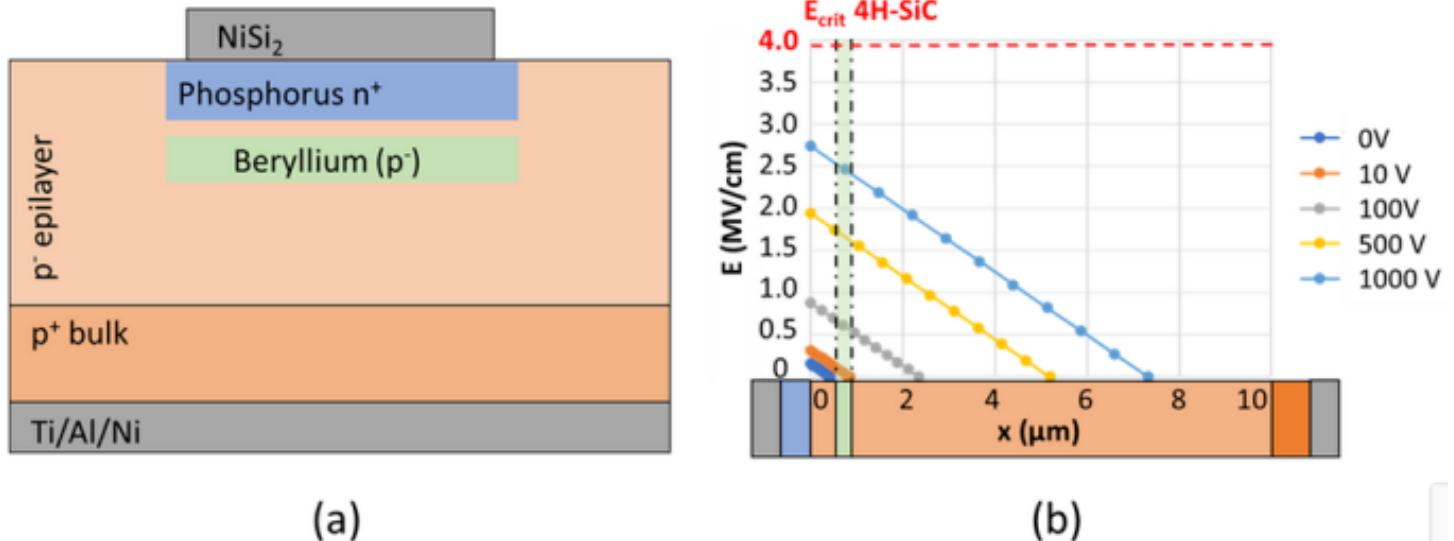
Figure WP2.1.1 layout of the devices used to constrain the NME of the  ${}^7\text{Be}$  decay (a); electric field in different positions of the epitaxial layer in different reverse bias conditions (b). In order to highlight the location close to the junction, the pictures in (a) and (b) are not in scale.
