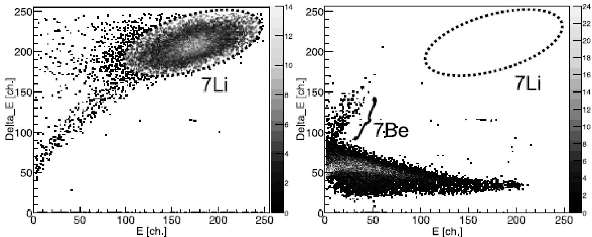
Fig. WP 1.2.2  $\Delta E/E$  matrices with a test  ${}^7\text{Li}$  beam (left) and a  ${}^7\text{Be}$  beam (right).  ${}^7\text{Li}$  spot is circled in the matrices.  ${}^7\text{Be}$  ions may channel through windows causing events on the left of the matrix.
