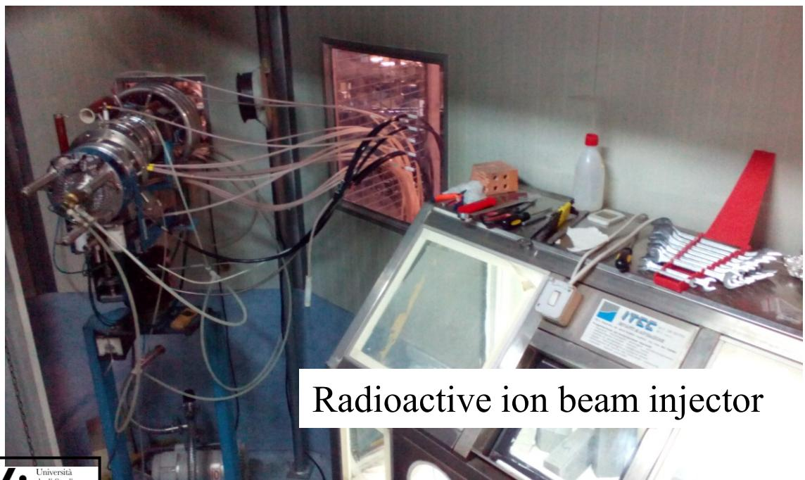
Radioactive ion beam injector
