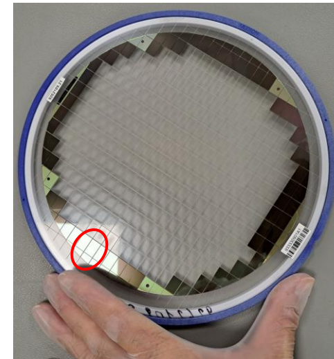
DarkSide-20K 8" wafer SiPM size: 8 \text{ mm} \times 12 \text{ mm} area: 96 \text{ mm}^2
