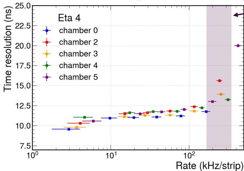
Time resolution of the chambers increases up to **15 ns @ 250 kHz/strip**
