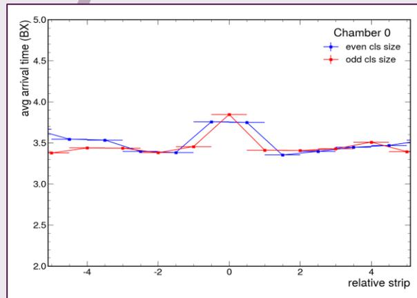
In the clustering process, the time of the cluster is taken as the one of the last firing strips
