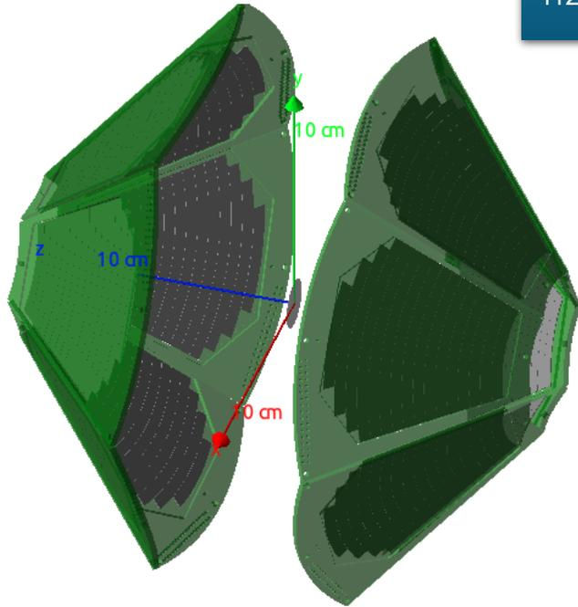
SIDAR array consisting of 2 lamp-shade SSD (12 YY1)
