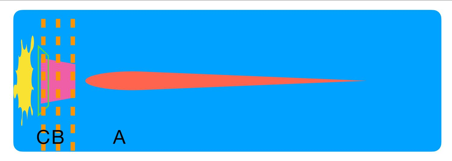
By keeping constant the z and the drift and transfer fields, and changing the GEM#1 gain, the total amount of electrons in the cloud increases and we should see only the effect of C: electrical repulsion within the electron cloud that depends, at least linearly, on it;
