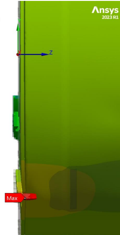
Figure 47: Insertion load case – Front Support deformation along Z direction.
