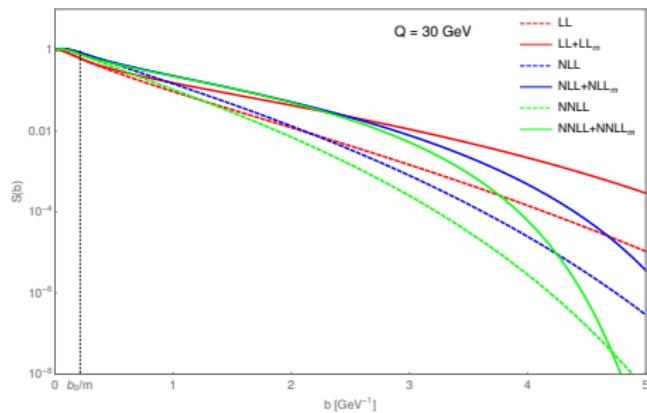
The massive Sudakov form factor  $S_m(Q, b)$  in  $b$ -space at a hard scale  $Q = 30$  GeV both in linear (left panel) and logarithmic (right panel) scales, at various logarithmic orders. The solid lines represent the massive case with  $m = m_b$ , while the dashed lines the massless case.
