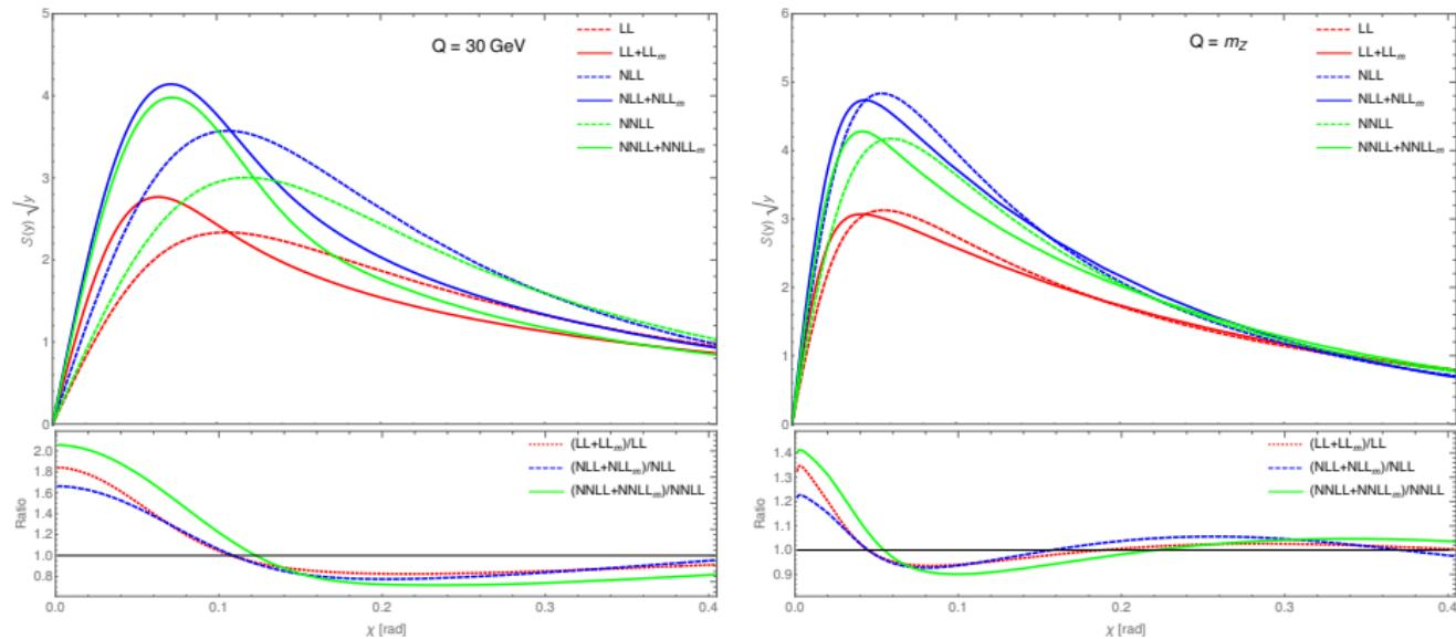
The massive Sudakov form factor  $S_{\uparrow\downarrow}(Q, y)$  in physical (angle- $\chi$ ) space for a hard scale  $Q = 30 \text{ GeV}$  (left) and  $Q = m_Z$  (right) in the massive case with  $m = m_b$  (solid lines) and massless case (dashed lines). Lower panel shows the ratio of the massive form factor over the massless one.
