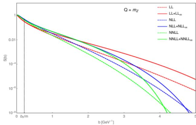
The massive Sudakov form factor  $S_m(Q, b)$  in  $b$ -space at a hard scale  $Q = m_Z$  both in linear (left panel) and logarithmic (right panel) scales, at various logarithmic orders. The solid lines represent the massive case with  $m = m_b$ , while the dashed lines the massless case.
