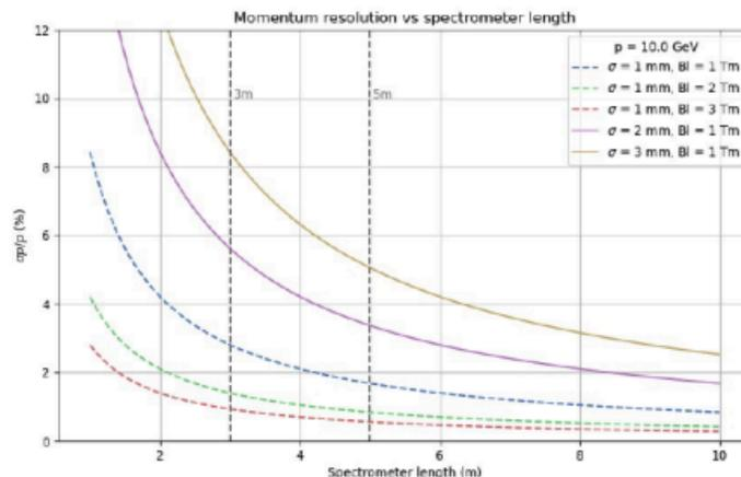
we can achieve a resolution  $\delta p/p < 1\%$  within a few meters of lever arm (depending on space constraints) for momenta up to a few GeV and with  $N = 10$  hit measurements
