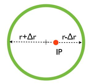
Moderate variation (+20%) according to FastSim in rates at L0 when moving the IP about 2 mm far in the XY plane from the nominal position. This is consistent with the naive expectation of null increase in case of linear approximation in a small interval  $\Delta r$  around r of the bkg rate vs r.
