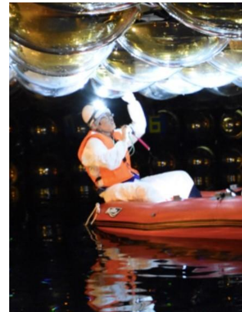
SK-V, 2019-2020 11,129 ID PMTs (refurbished for Gd and with Hyper-K PMTs)
