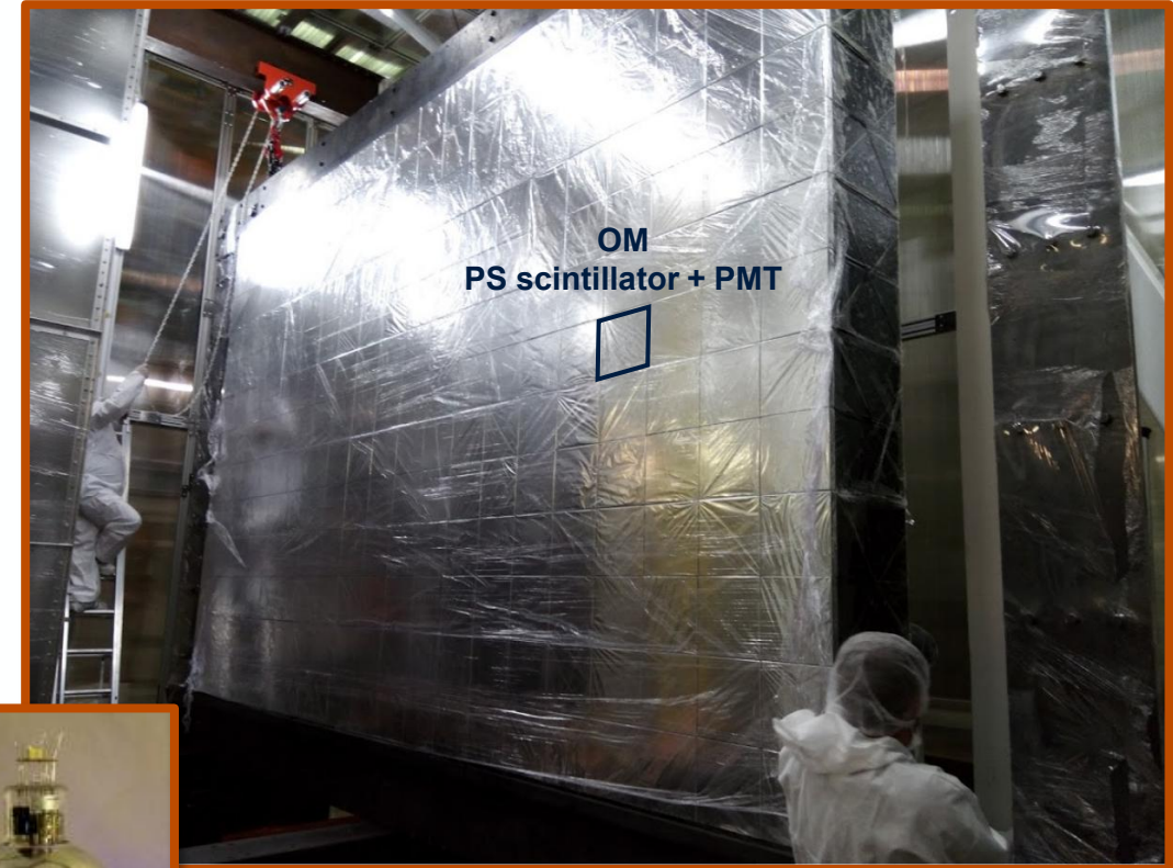
Calorimeter main wall ( 6 \times 4 \text{ m}^2 )
