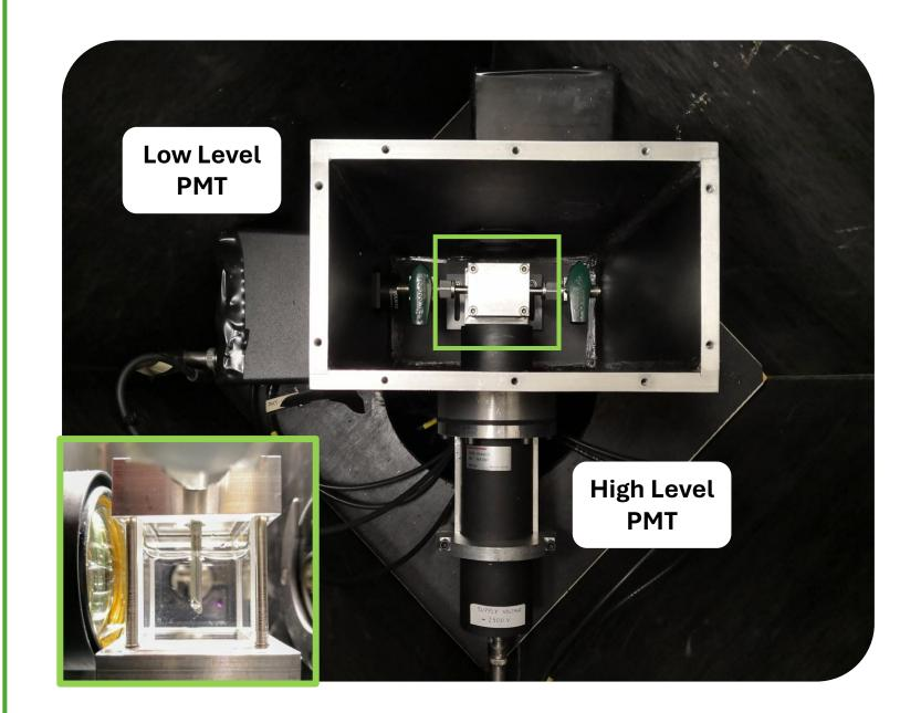
The knowledge of the fluorescence time profiles of the scintillator via small-scale setups are fundamental for JUNO: both for position and time reconstruction, but also for particle identification through the Pulse Shape Discrimination.
