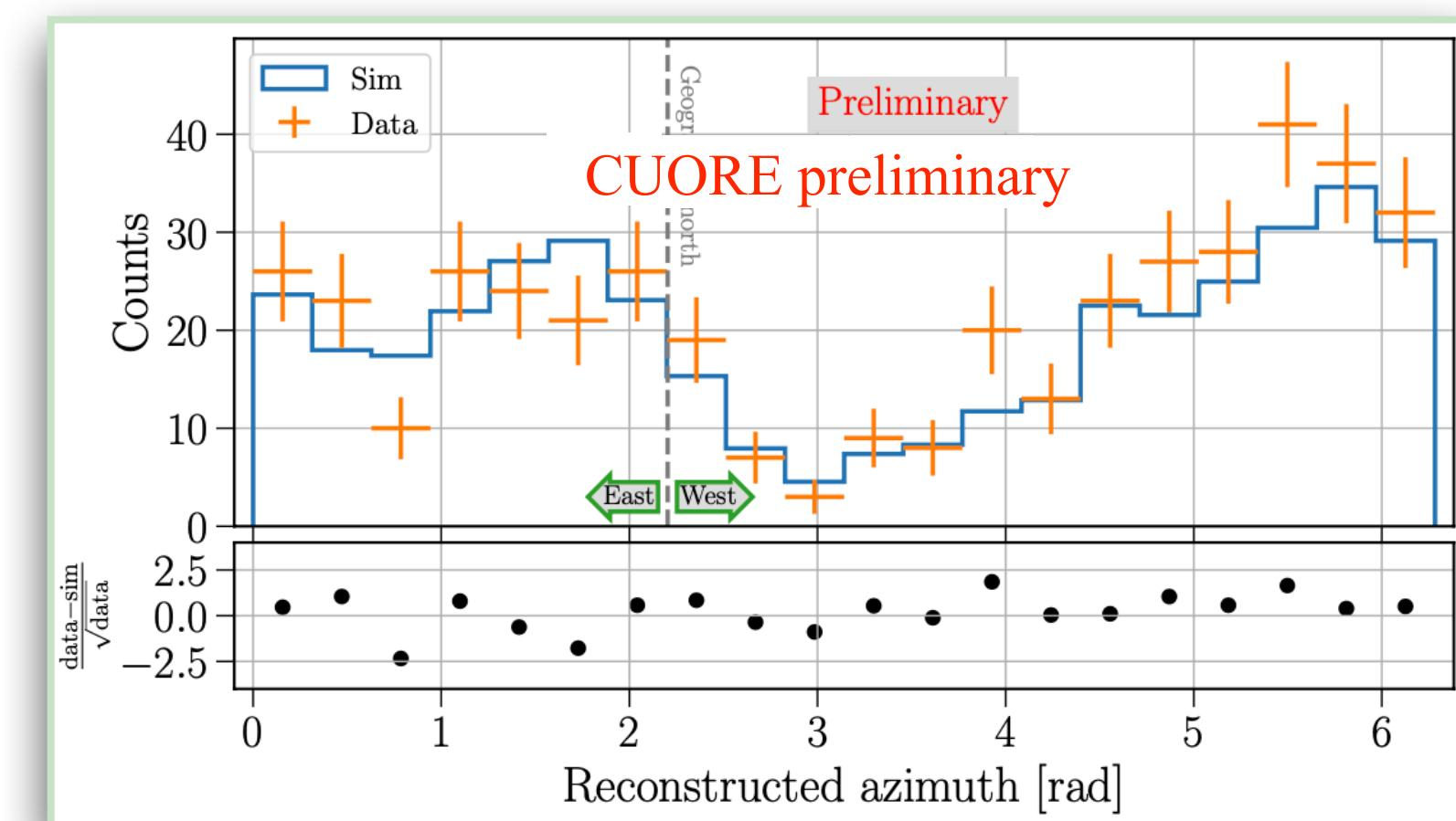
Track-like events ( $N_{\text{crystals}} \geq 5$  &  $E_{\text{dep}} \geq 9$  MeV) to study  $\mu$ -induced background
