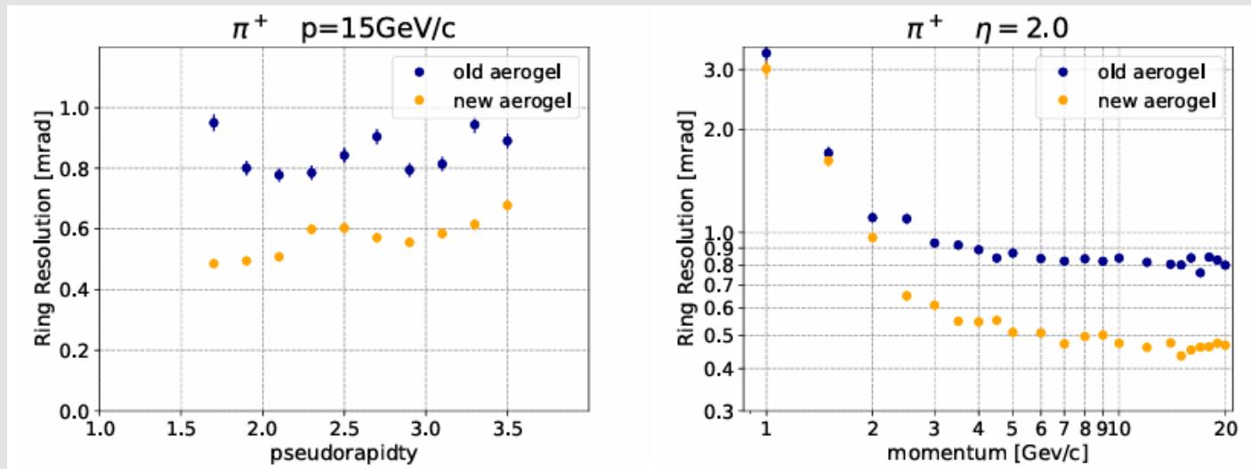
New type-1 Aerogel provides ring resolution capable to perform PID  $\sim 18\text{-}19 \text{ GeV}$  (@ $\eta=2.0$ ), baseline aerogel is limited only upto  $15\text{-}16 \text{ GeV}$
