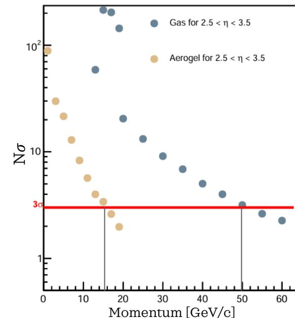
@  $\eta > 2.5$  we achieve 3 $\sigma$  with  $\sim 15$  GeV/c of momentum for the aerogel and  $\sim 50$  GeV/c for the gas.
