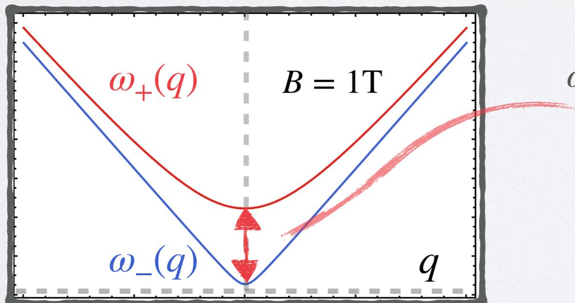
$$\begin{aligned} \omega_{\alpha=\pm}^2(q) &= \mu^2 B^2 + \lambda_x + 2\lambda_z + v_\theta^2 q^2 \\ &\pm \sqrt{4\mu^2 B^2(\lambda_x + 2\lambda_z + v_\theta^2 q^2) + \lambda_x^2} \end{aligned}$$
