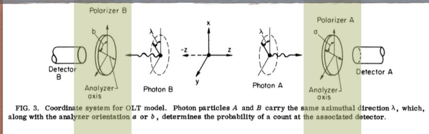
FIG. 3. Coordinate system for OLT model. Photon particles A and B carry the same azimuthal direction  $\lambda$ , which, along with the analyzer orientation  $a$  or  $b$ , determines the probability of a count at the associated detector.
