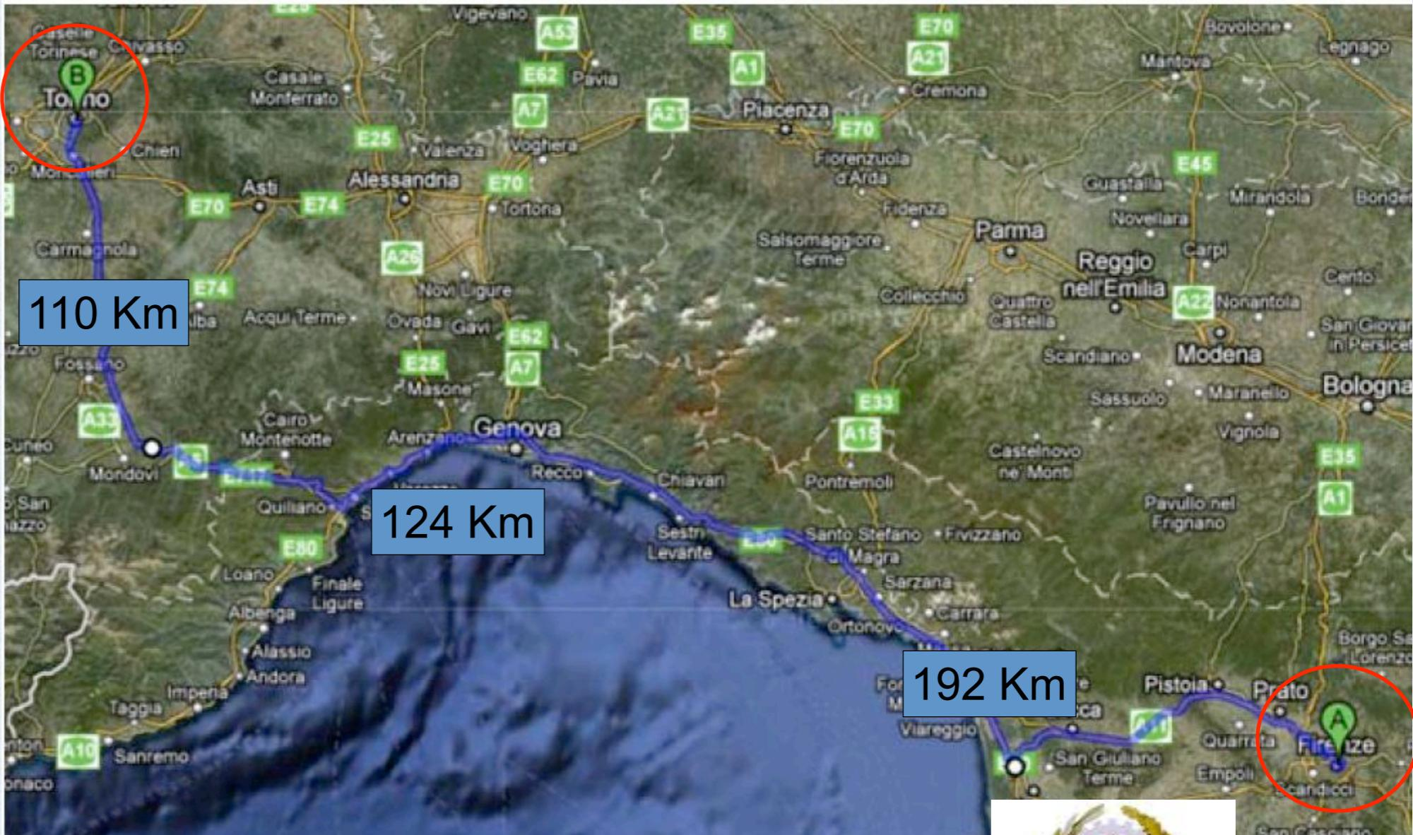
430 km link : two EDFAs, two  $1.5 \mu\text{m}$  laser
