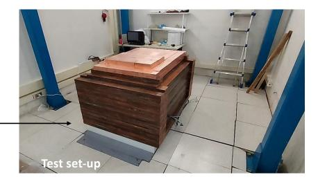
A new SABRE test set-up was installed in the new area. Dimensions  $\approx 1.7 \times 1.4 \times 1 \text{ h m}^3$  Capable to host up to 2 crystal enclosures per time. The construction of a new Rn-box in Lexan is in progress.
