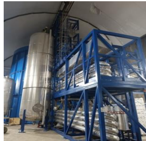
Gas stripping to remove Rn and O 2
