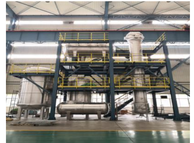
Water extraction to remove radioactive impurities
