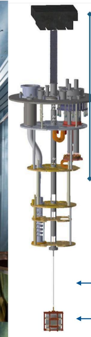
Spring-pendulum hanging from independent rack and thermally coupled to 4K stage
