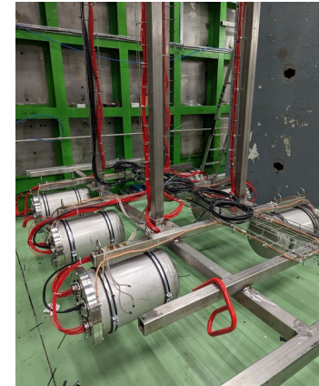
Electronic vessels at the under water test facility at CERN
