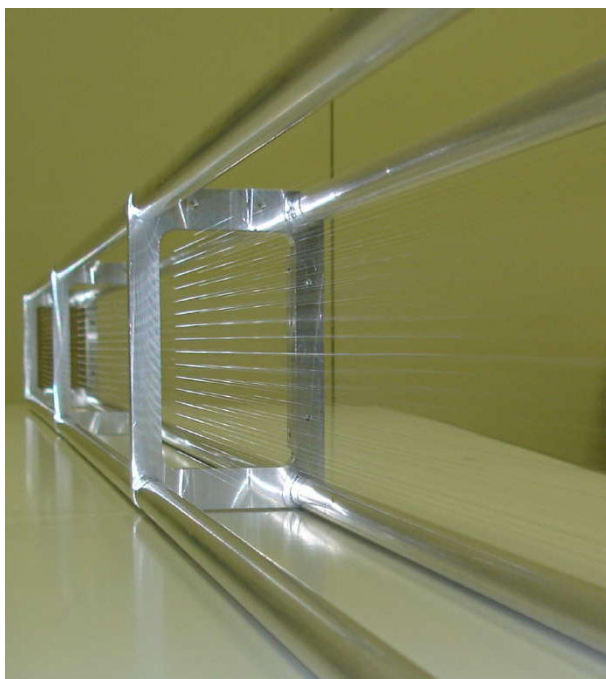
Figure 1.11: Prototype 2: detail of the strung wires.
