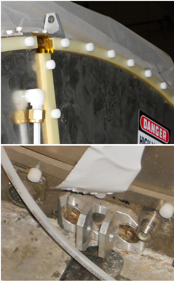
Figure 1.33: Mechanical mounting points for the BABAR dch on the (a) forward and (b) backward ends. Both ends are attached to the DIRC central support tube.
