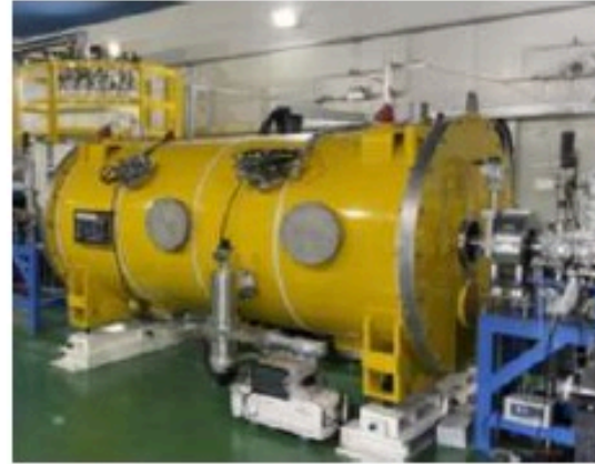
CEPC collider ring 650MHz 2*cell short test module has been completed in TDR phase
