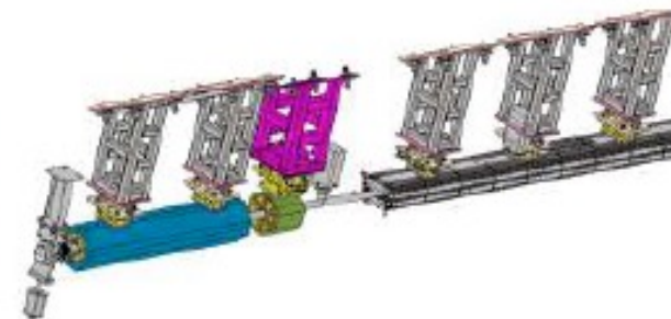
Booster magnets installation
