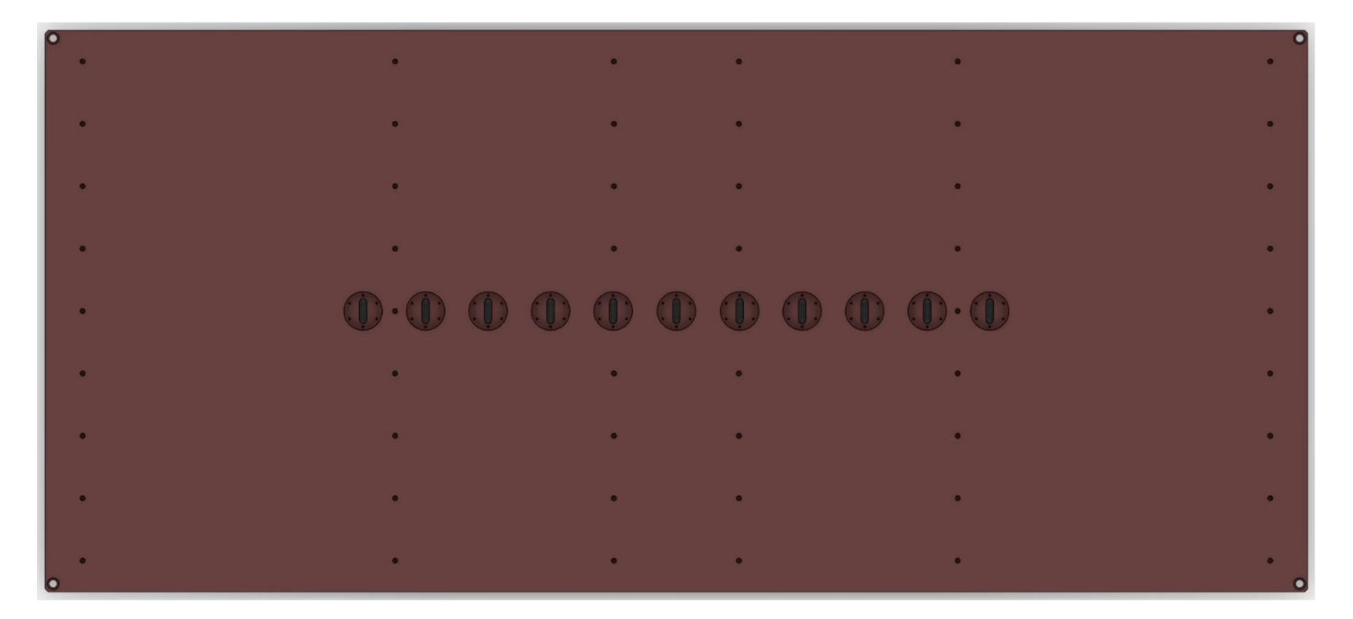
In the pure copper there will be 14 (11 in the picture) slits, where the source will be exposed
