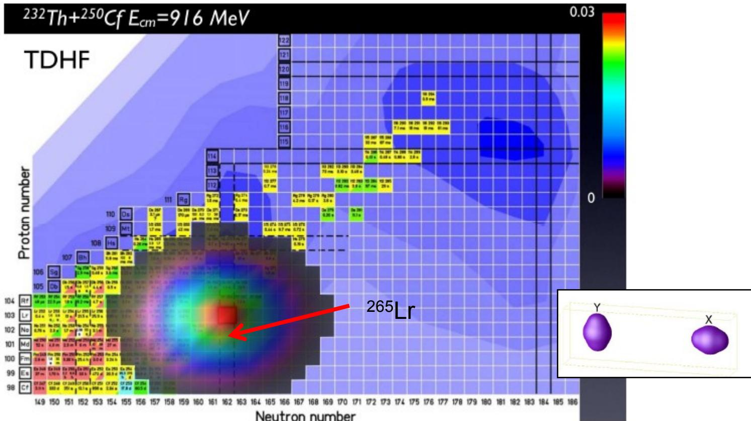
TDHF probability distribution for the heavy fragment produced in  $^{232}\text{Th} + ^{250}\text{Cf}$  central collision in the  $xy$  configuration.
