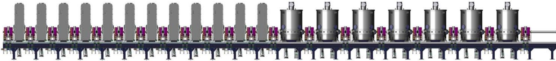
12 low beta cryomodules (0.07) and 7 high beta cryomodules (0.12)
