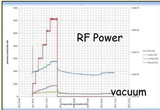
RF long duration tests at 6 kW
