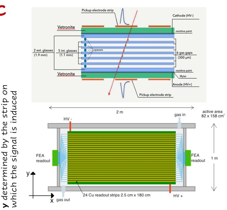
$\boldsymbol{x}$  determined by measuring the difference between the arrival time of the signal at the two ends of the strip
