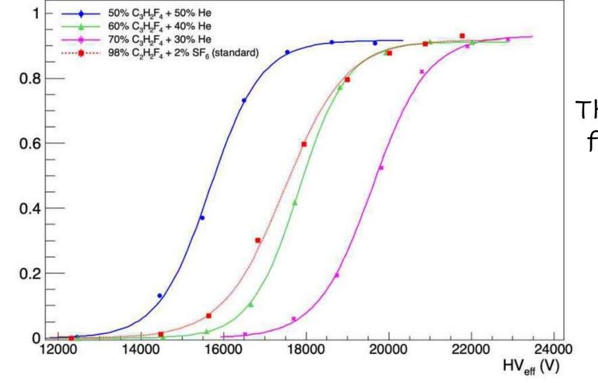
The chambers are filled with an eco gas mixture  $C_3H_2F_4 + He$ with  $GWP (\sim 6)$
