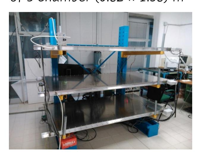
Each chamber has six 300  $\mu$ m gas gaps with 24 readout copper strip electrodes (180 cm x 2.5 cm spaced by 7 mm)
