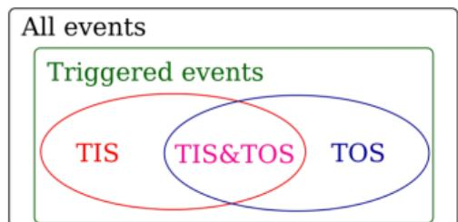
Figure 1: Diagram explaining the logic behind categorizing events into Trigger On Signal (TOS), Trigger Independent of Signal (TIS) and Trigger On Both (TOB) trigger categories. Note that an event can be both TIS and TOS simultaneously.
