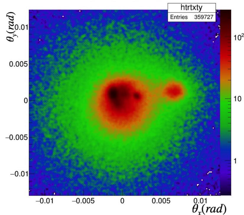
Beam core structure clearly visible with passing-through tracks
