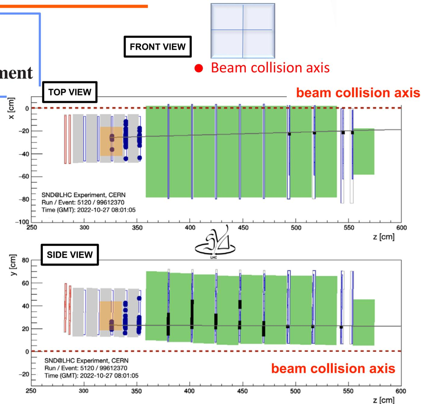
FIG. 2. Display of a  $\nu_\mu$  CC candidate event. Hits in the SciFi, and hadronic calorimeter and muon system are shown as blue markers and black bars, respectively, and the line represents the reconstructed muon track.
