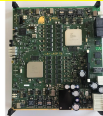
LAr Signal Processing (LASP) demonstrator under testing
