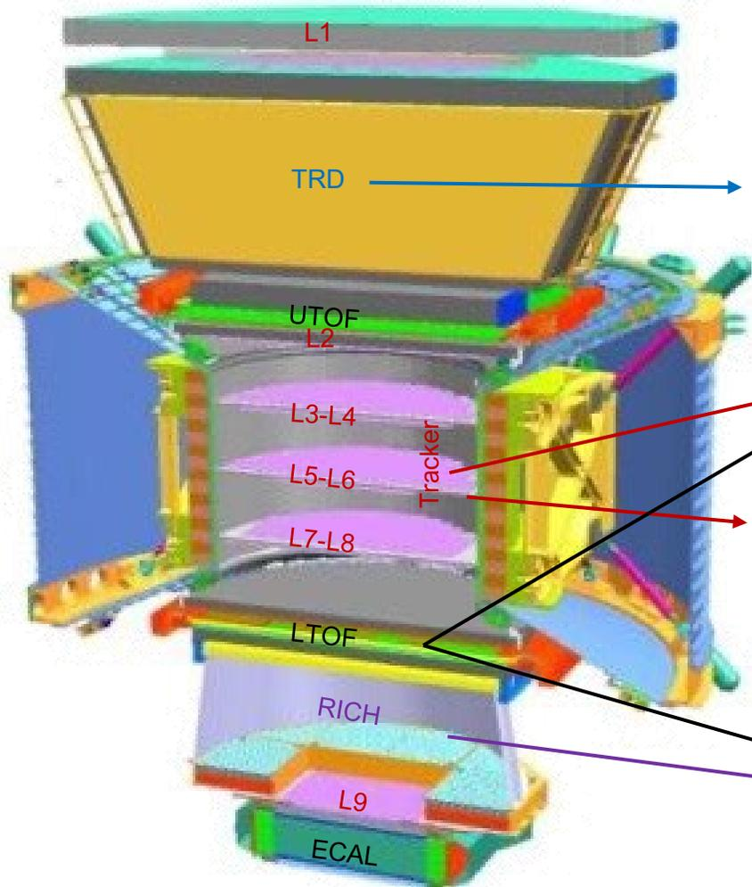
The **TRD** helps with the particle identification.
