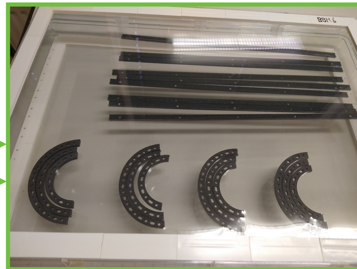
Half-rings thickness moved from 6 mm to of 3 mm → Logerons length moved from 251 mm to 256 mm
