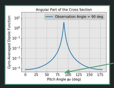
**Maximum** sensitivity occurs when the **Observation Angle** matches the RE Pitch Angle
