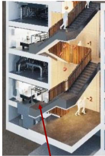
Laser lab for AION vibration criterion, VC-G = 10nm@10Hz. Temperature (22±0.1)° C
