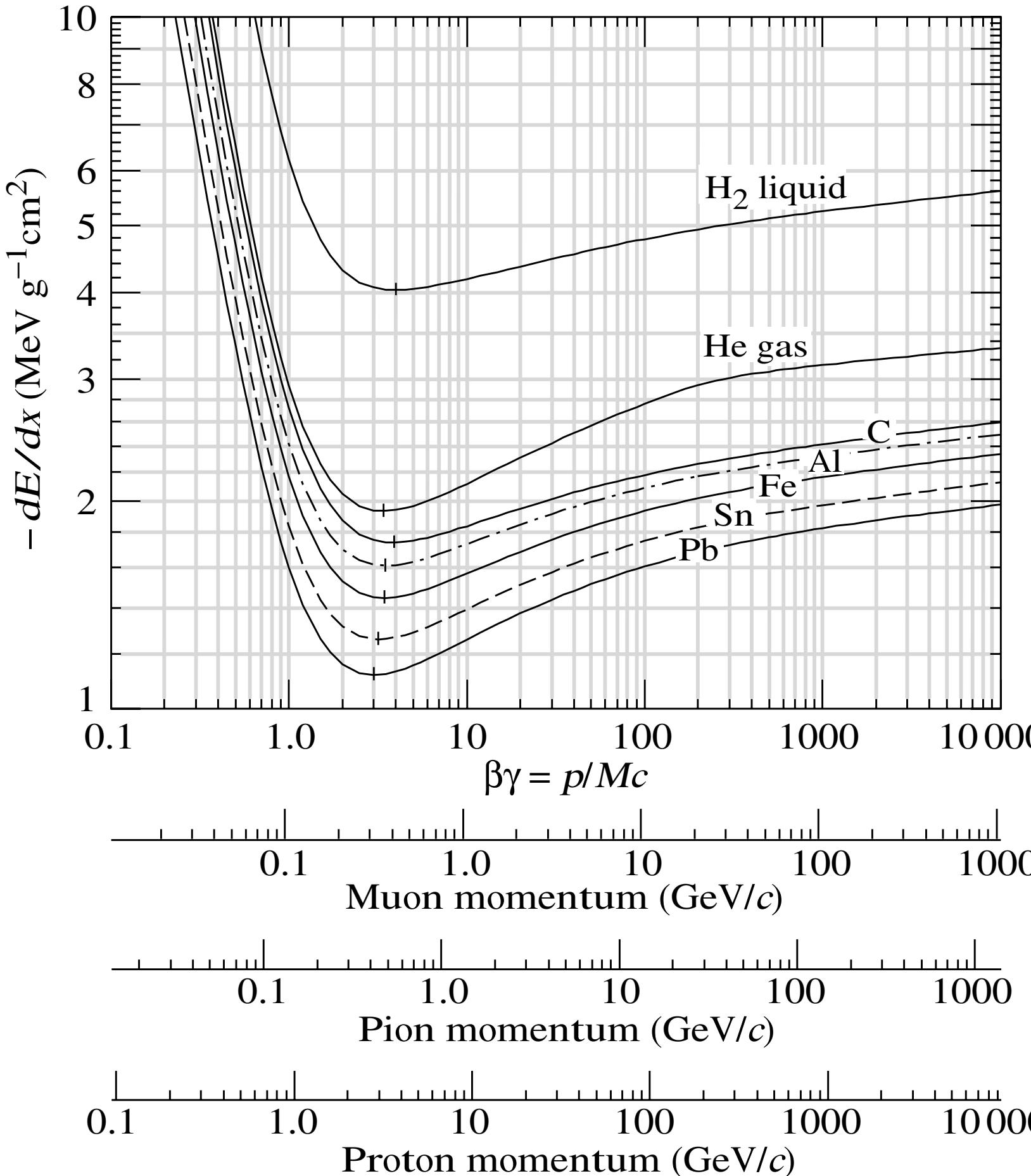
$$-\frac{dE}{dx} = K z^2 \frac{Z}{A} \frac{1}{\beta^2} \left[ \frac{1}{2} \ln \frac{2m_e c^2 \beta^2 \gamma^2 T_{\max}}{I^2} - \beta^2 - \frac{\delta(\beta\gamma)}{2} \right]$$
