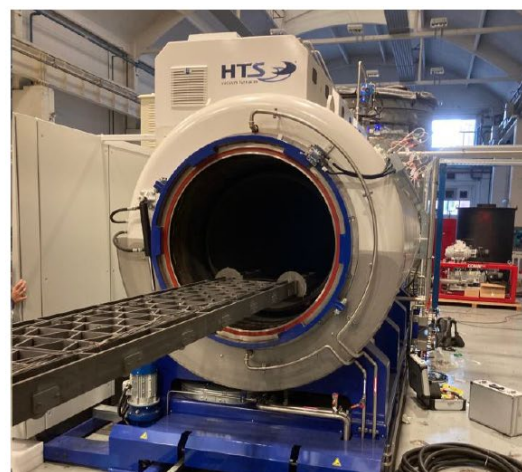
Furnace for coil heat treatments
