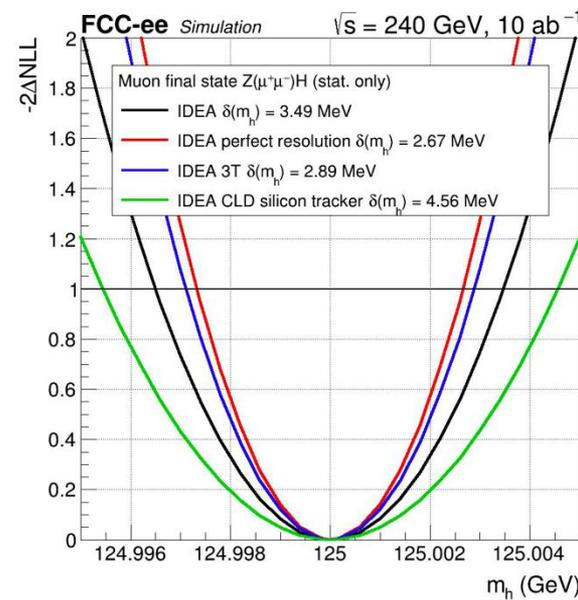
$\mu$  from Z, with momentum of O(50) GeV, to be measured with a  $p_T$  resolution smaller than the BES in order for the momentum measurement not to limit the mass resolution
