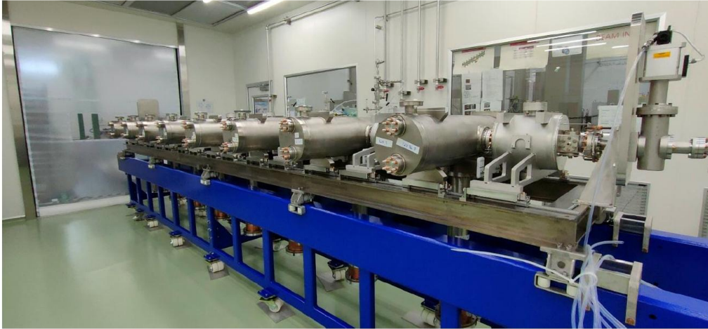
Picture 2-3: Beam line fully assembled
