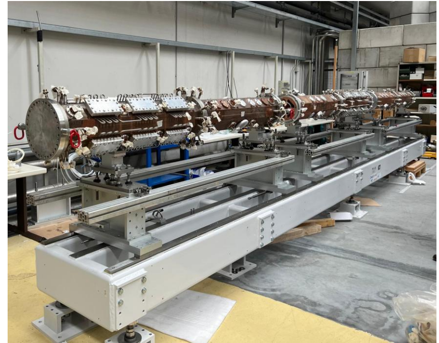
Anthem RFQ to be transported on the support assembled to Caserta after tuning and vacuum leak checks. (CW, 600kW, 352MHz)
