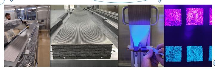
Module ready for fiber insertion Scintillating and Cherenkov fiber batches prepared for PMT integration
