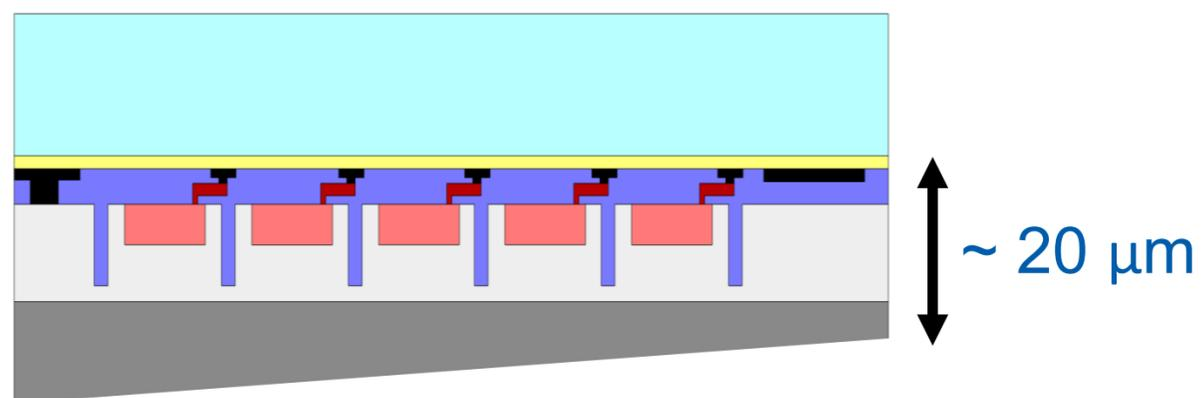
Remaining Substrate buffer after grinding: ~ 20  $\mu\text{m}$
